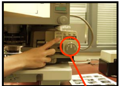
Press the button marked "Load/Rew". Turn knob right for forward and left for reverse. Return knob to center to stop.
